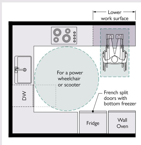
Figure 15: U-shaped kitchen, from CMHC Accessible by Design Guidance (2016).
