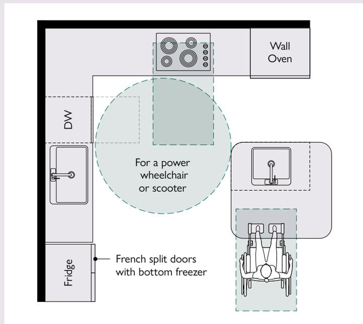
Figure 14: L-shaped kitchen, from CMHC Accessible by Design Guidance (2016).
