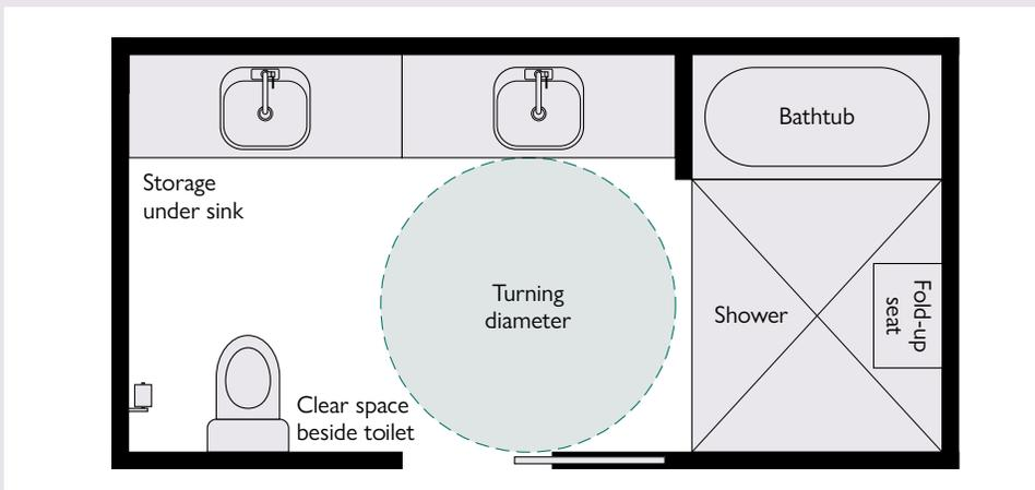
Figure 10: Bathroom with curbless shower and bathtub, two wash basins, toilet, and storage space. Adapted from CMHC, 2016.
