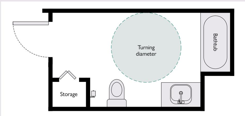
Figure 9: Small, widely usable, and accessible bathroom. Adapted and amended from CMHC, *Accessible Housing by Design—bathrooms*, 2016.
