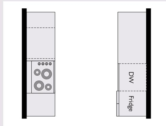
**Figure 16: 1,800-mm floor space for a galley-style kitchen, from CMHC Accessible by Design Guidance (2016).**
