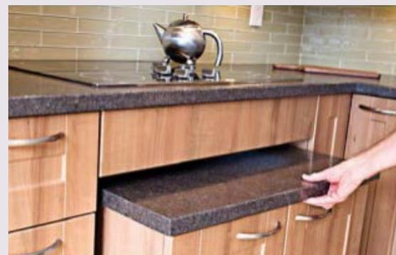
**Figure 18: Rolling cabinet provides legroom under cooktop and is a portable workstation.**
