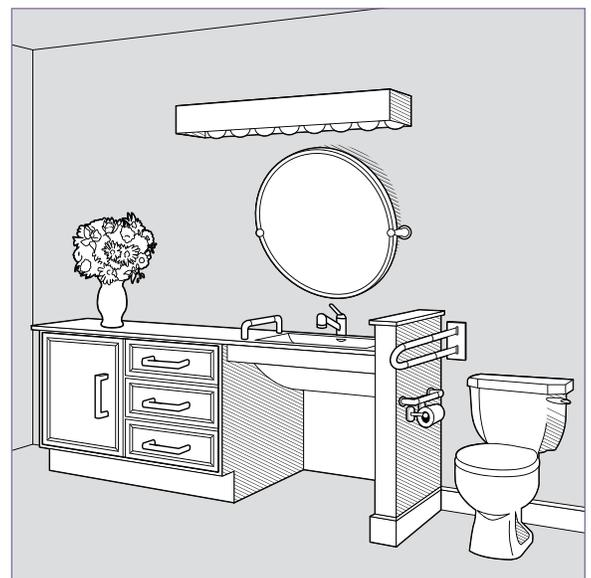
**Figure 15:** The mirror should be positioned at a convenient height, and tilted if necessary, so that it can be used from a standing or a sitting position. Grab bars by the sink can provide additional stability.
