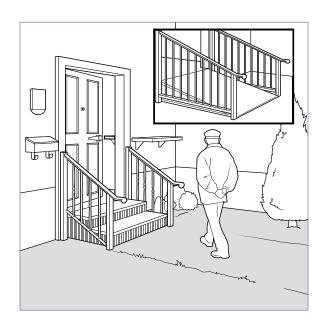
Figure 3: Low thresholds, small ramps or extra steps with a handrails or grab bar can be used at changes in floor levels in door openings.
