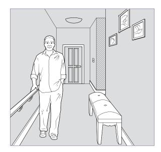
**Figure 7:** Handrails along corridors help people with poor balance or mobility. Seating in a corridor gives people a place to rest.
