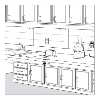
Figure 13: Install electrical outlets so that small kitchen appliances can be used in convenient locations without being moved.
