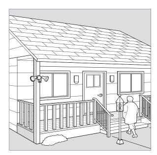
Figure 2: Well-lit walkways, steps and entrances, as well as colour contrasts, help people with low vision to detect obstacles. Ensure lighting does not cast shadows on steps.
