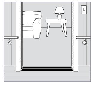
Figure 6: Strong colour contrast strips or changes in floor texture can help people with low vision detect possible obstacles when moving between rooms.
