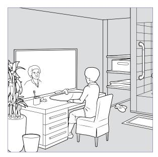
Figure 14: If you tend to lean, pull or push against the basin, it may need to be supported on legs or a solid cabinet. A cabinet can be designed to allow you to use the basin from a seated position.
