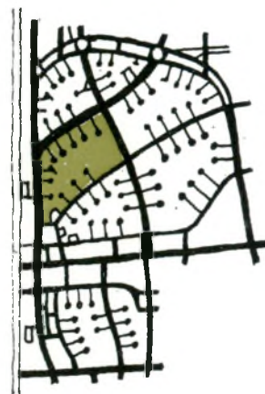
1 The original traffic separation layout at Radburn, New Jersey. (left) One of the completed neighbourhoods, (right) the block plan.
