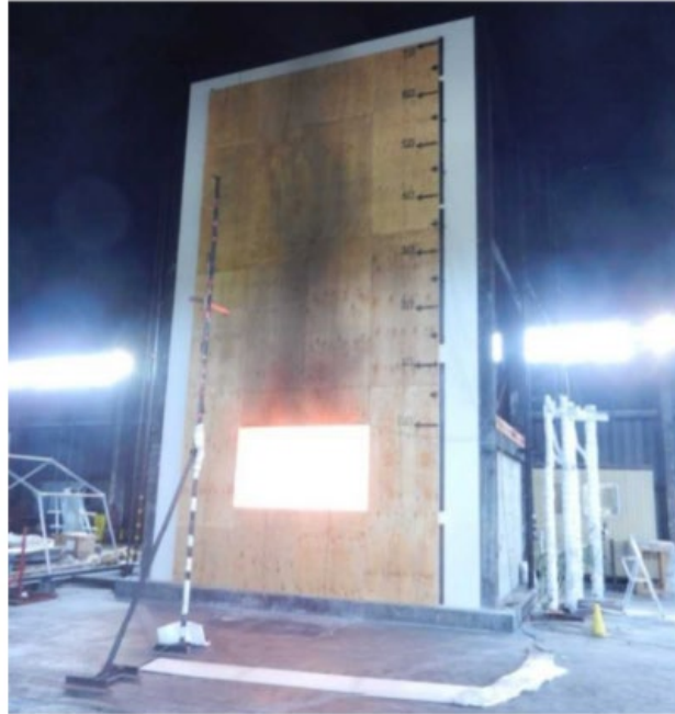
Figure 30. CAN/ULC-S134 full-scale test of exterior wall assembly (Su & Lougheed, 2014).
