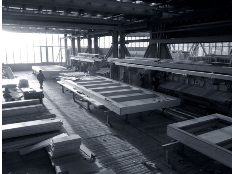
Figure 23. Fabrication of facade panels (courtesy of CREE).
