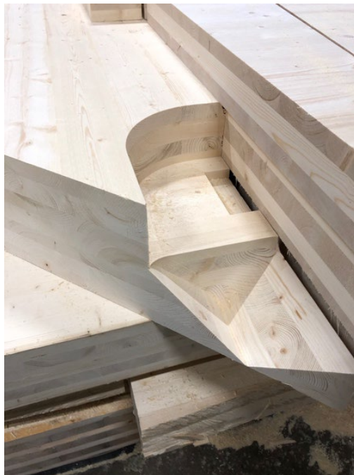
Figure 2. Precisely processed CLT panel, Hoisko CLT Finland Oy (courtesy of Mark Taylor).
