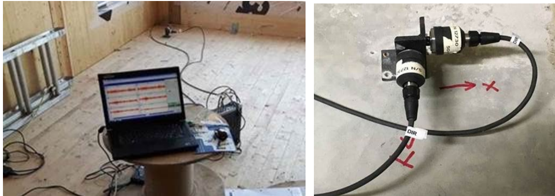
Figure 3. Vibration testing being conducted in a building (left: indoor setup; right: accelerometer sensors).
