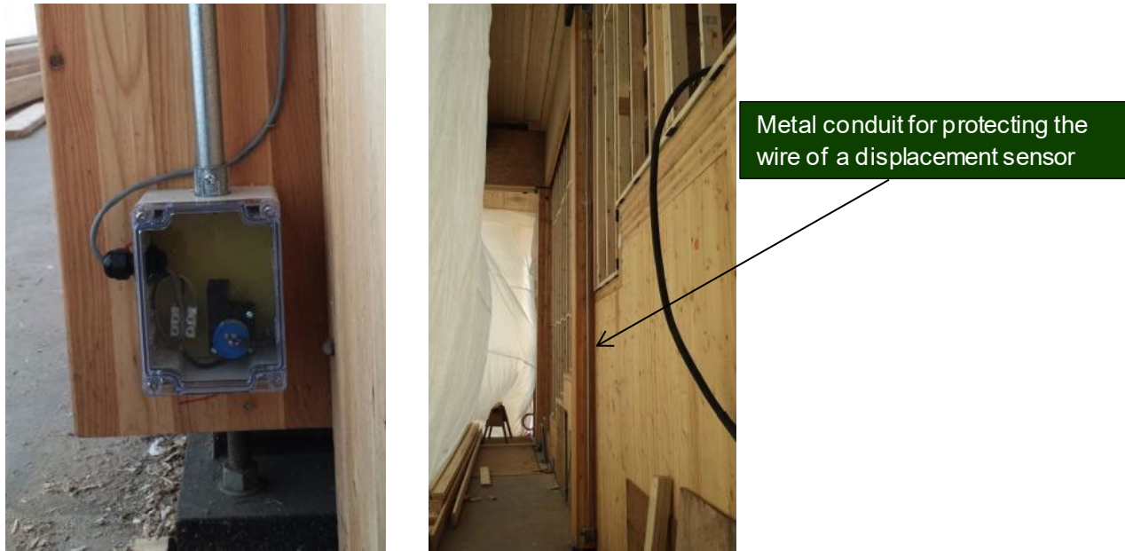
Figure 10. A displacement sensor (left: the sensor box, which is adjacent to the column base; right: its metal conduit for protecting the wire) installed for measuring the vertical movement of a glulam column (Wang, 2018).
