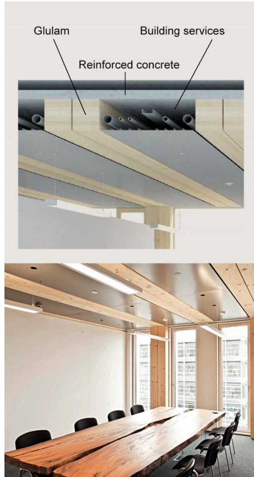
Figure 20. Service integration between beams (courtesy of CREE).
