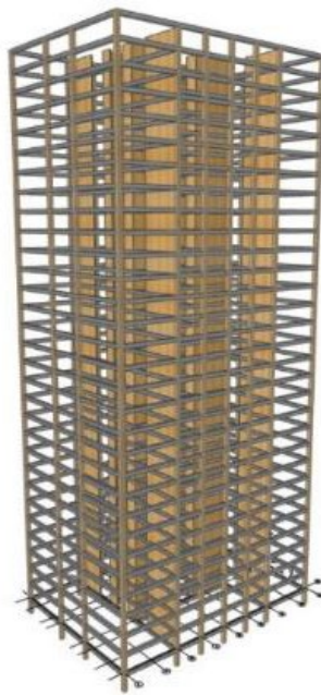
Figure 22. 3D view of the 30-storey mass timber building (Bezabeh et al., 2020b).
