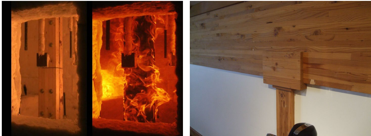
(a) Fire-resistance test conducted on concealed plate (courtesy of L. Peng, 2010)
