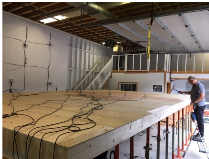
Figure 4. Vibration testing of a mass timber floor at FPInnovations.
