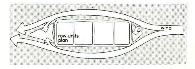
Unit expanion should occur in a row parallel to the direction of the prevailing cold winter winds.
