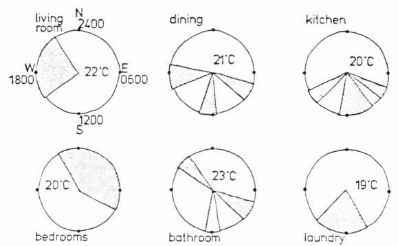
Provide each area with maximum solar impact for the period during which it is occupied.
