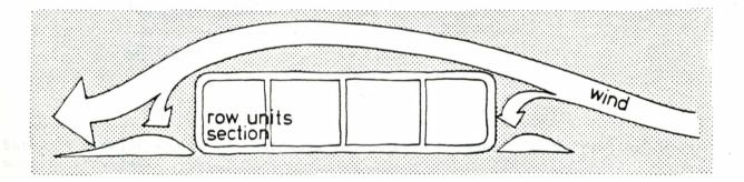
Simplified building form and lower height to width ratio provide a profile which minimizes heat loss and snow accumulation.
