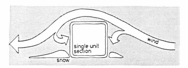
The cubic housing form has been found to be the most efficient, practical shape in minimizing heat loss in winter and heat gain in summer. There is also less snow accumulation around simple forms which offer little wind resistance. Thus the ideal detached house form should be the most compact (cubic) shape with minimally exposed exterior surfaces.
